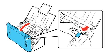
4. Gently pull out any jammed originals from inside the scanner.
